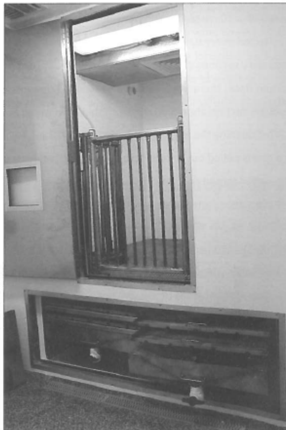
Figure 2. Calorimeter chamber with the fecal screens and urine collection pans under the slatted floors
