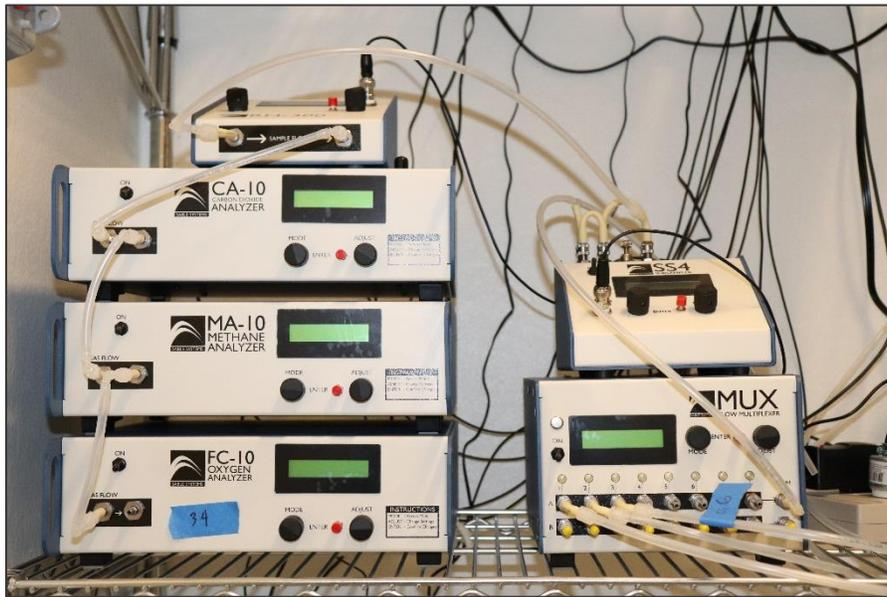
**Figure 3.12.** Gas analyzers system.
