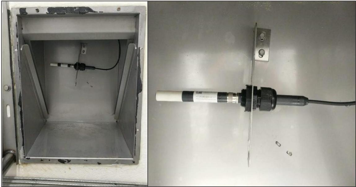
**Figure 3.14.** Temperature and humidity sensor.
