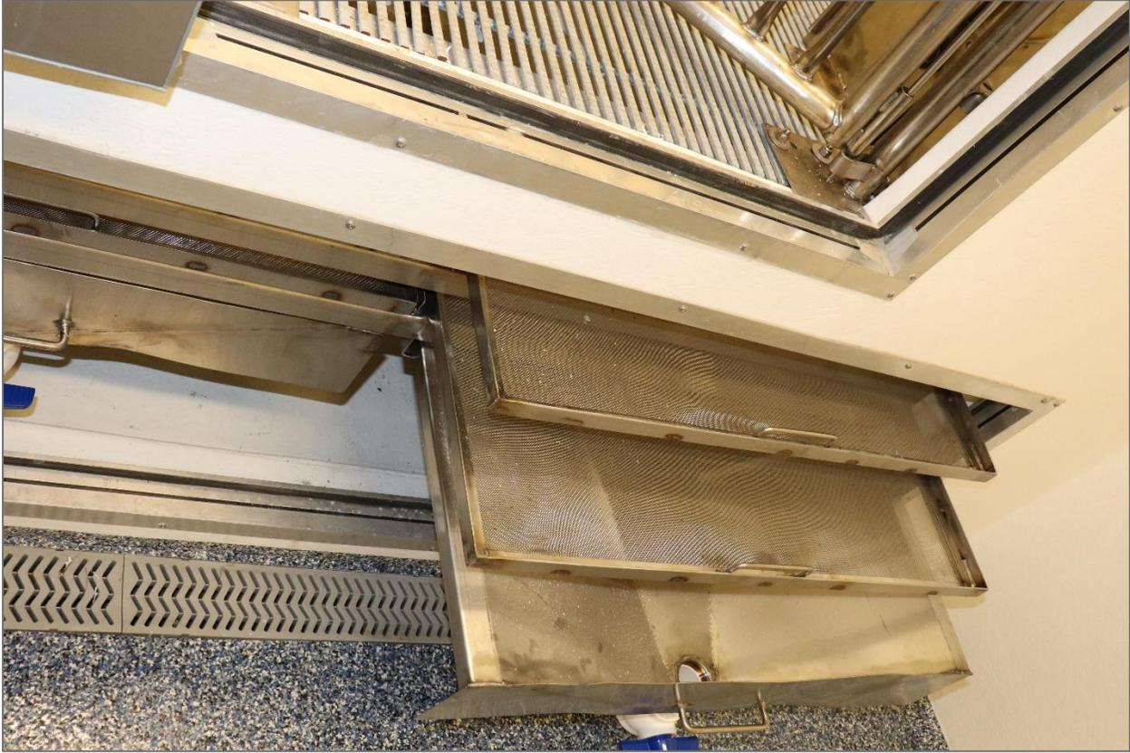
**Figure 3.8.** Screens and urine pans inside the secondary section of the calorimeter chamber.
