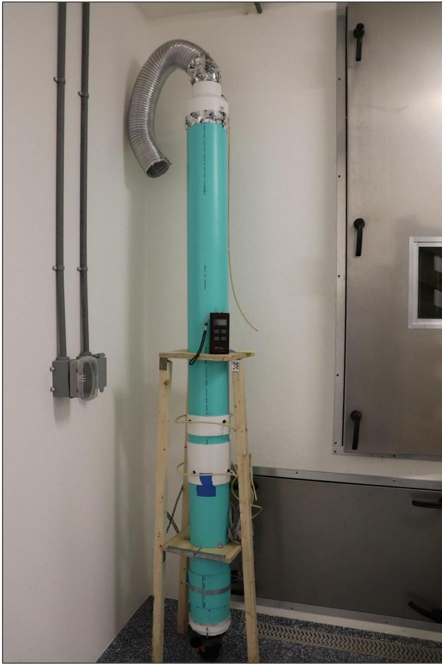
**Figure 3.13.** Fresh air supply system calibrator.
